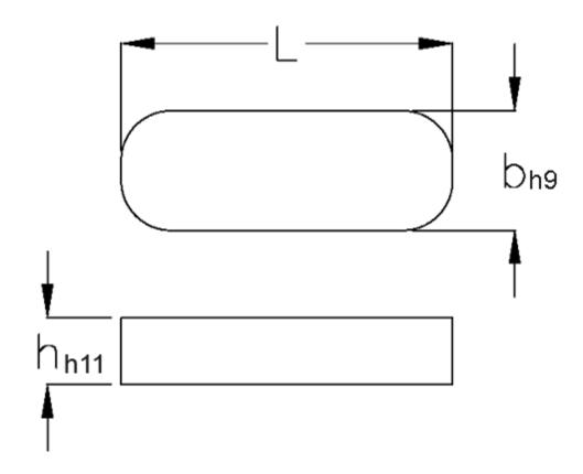
b = 12 h = 8 L = 80.0 Tolerance b = 0.043 Tolerance h = 0.090 Tolerance L = -0.3
